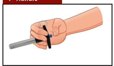
The T-handle allows for a strong grip from the two extensions on either side. This handle works well when you have room for the handle and you need a firm grip.
