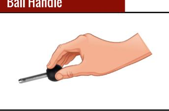
The ball style handle is not activated by the push of a button. They allow a firmer grip on the detent pin and are good for small spaces. They can help prevent accidental removal because nothing can get snagged, unlike the ring style where something could get caught in the ring and pulled out.
