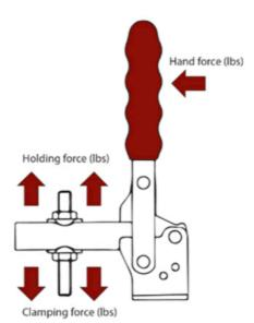
Clamping Force - That which will result from the quoted hand force. Clamps with a fixed clamping position have a single clamping force quoted. Those where the threaded spindle may be positioned at any point along an arm (arm type B) and those with solid arms to be cut and welded as required (arm type A) have clamping forces quoted at the inner and outer ends of the arm.
