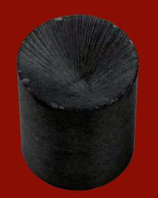
Ceramic magnets are also referred to as Ferrite magnets. The ceramic magnet is a nonmetallic compound of pure grades of iron oxide and strontium carbonate, and small quantities of other metal oxides. There are two different ways to make these magnets by pressing or sintering.
