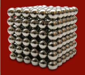
Neodymium Iron Boron magnets are a type of rare earth magnetic material. These magnets are known by a few different names. It can be seen as NdFeB because it is made from an alloy of these three different materials.
